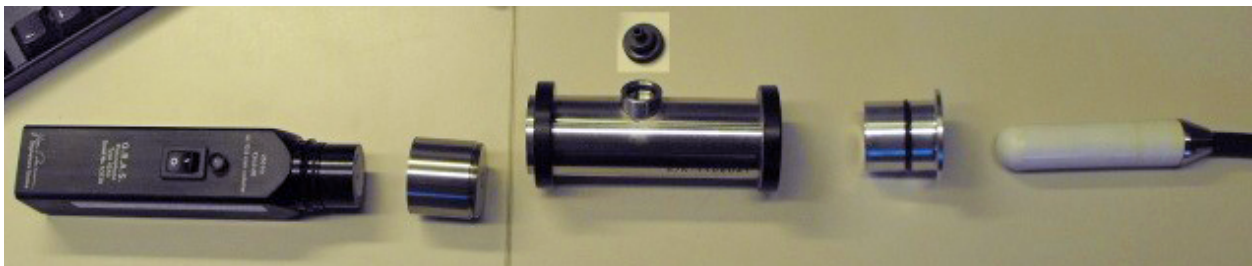
Figure 9. Split view of a G.R.A.S. 42AC pistonphone calibrator with an M15B hydrophone.
