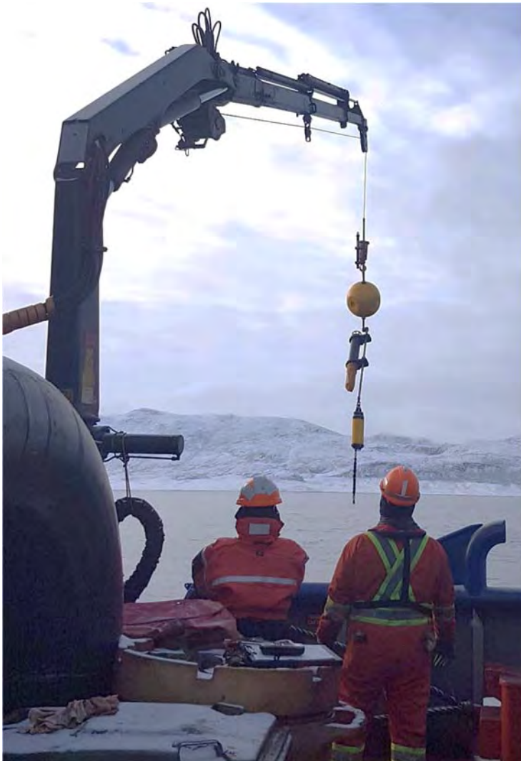
Figure 4. The Autonomous Multichannel Acoustic Recorder (in the middle of the mooring - AMAR G3; JASCO) used to measure underwater sound in and near Milne Inlet.
