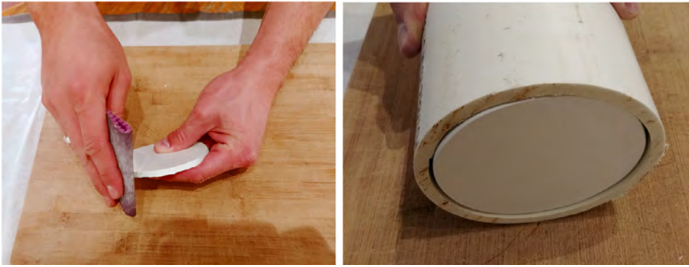
Fig. 18. Sanding edges of the discs.
