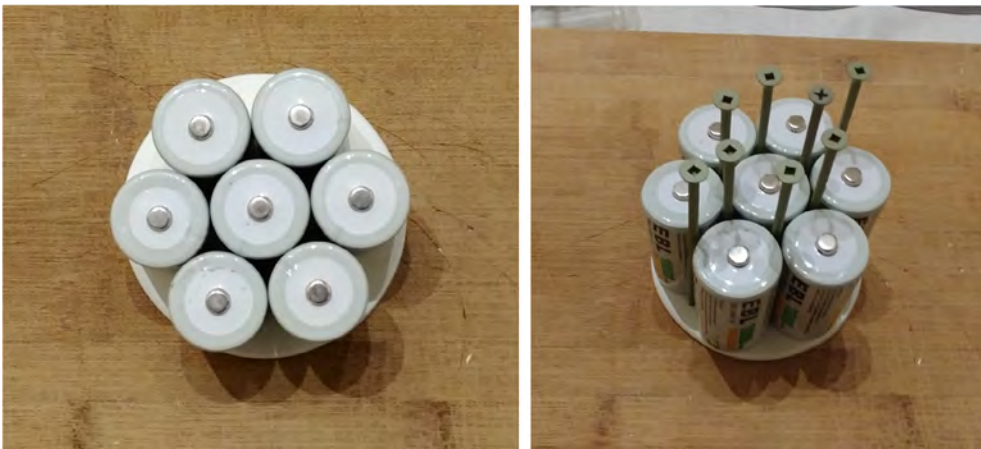
Fig. 19. Locating holes to drill on the discs.
