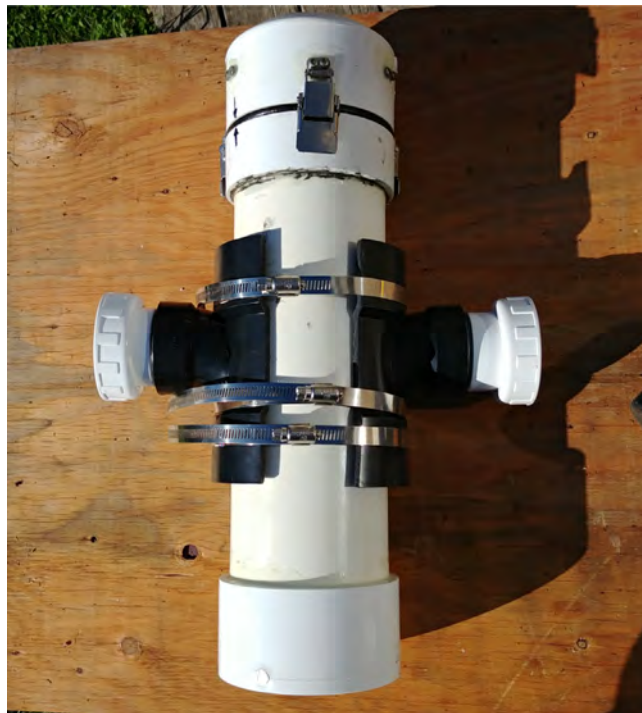
Fig. 34. Installation of PVC attachments to the pressure housing of the Fishcam.
