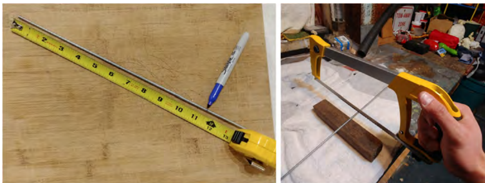
Fig. 22. Cutting of the metal rods.
