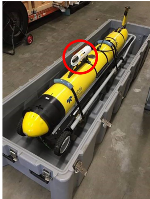
FIG. 1. (Color online) Teledyne Webb Research's generation-3 Slocum glider with a top-mounted hydrophone (circled in red) before deployment in the Gulf of St. Lawrence.
