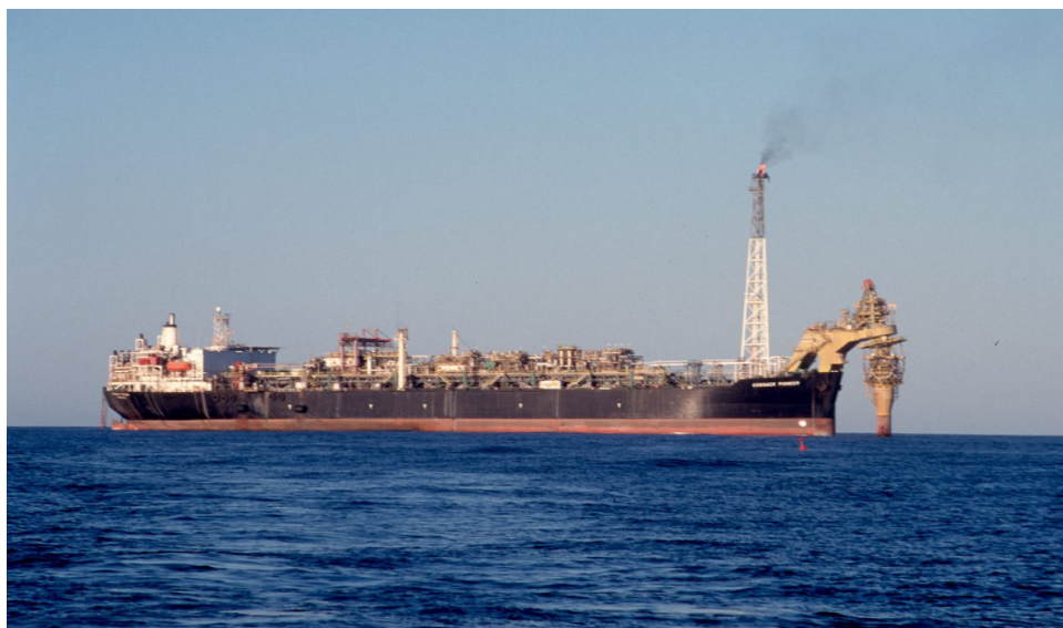
Fig. 1. (Color online) Photo of the Cossack Pioneer FPSO (bow attached to riser on the right side of the picture).
