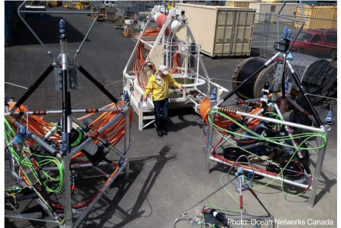
Acoustic and oceanographic sensors for the VENUS ocean observatory in British Columbia, Canada: Two JASCO Observers with tetrahedral hydrophone arrays
