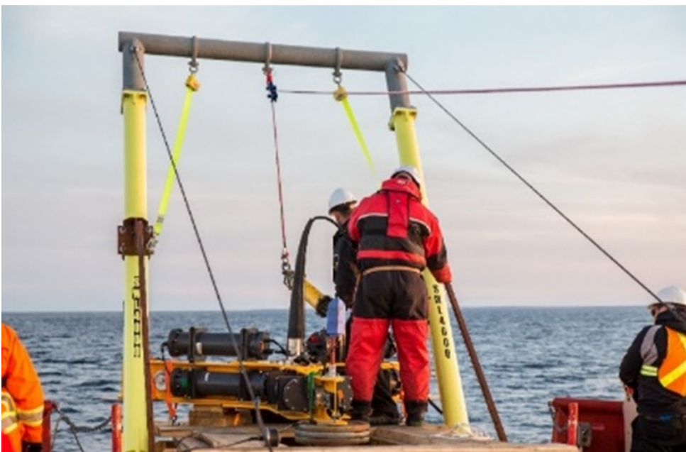
The OceanObserver Spar Buoy with bottom lander can be deployed from smaller vessels than large, open-ocean discus buoys
