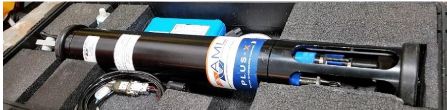
Figure 6. Minos Plus X used for CTD casts at the three AMAR sites.
