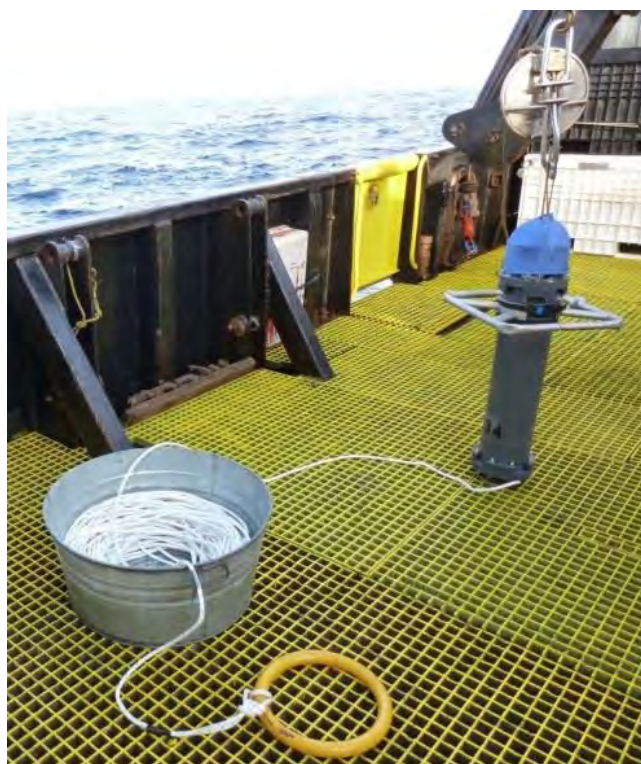
Figure 2. An AMAR just before it was deployed in the northeastern Chukchi Sea.
